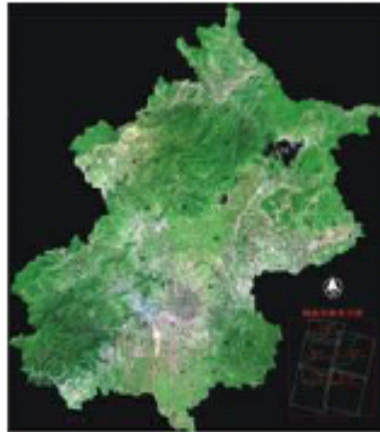
Mosaic image of Beijing with 5 scenes of CCD images, R3G4B2 pseudo color composite
